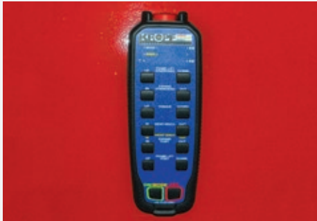
Wireless radio remote control with manual backup
